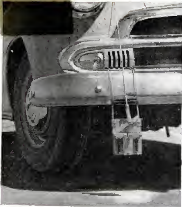
Detonator on front bumper fires chalk on road when signal to stop is given. It fires a second mark when brakes are applied, showing reaction-time travel
